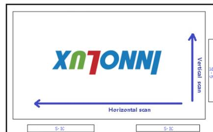
Fig. 2 Reverse scan (Pin24, Reverse = High)
